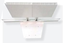
This Baseplate is made with a channel into which the panels fit and a platform welded behind which the Ballast Bottle Weight sits on to provide the counterweight and prevent the wall from overturning. The Baseplate is made out of sheet metal and has two rectangular section vertical rods welded within the channel that are designed to occupy the second cell on either end of every panel. There is a non-slip rubber matting below the platform helping to keep the Baseplate in position.
